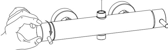
By changing the output selection results in dripping from both ways as a safety feature, in way to not forget the mixer in open position and avoid exposing the diverter to unsuitable pressures.
